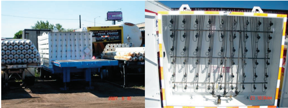
54 3AA - 2400+ PSI cylinder trailer - in test to July 2012
